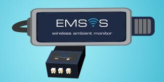
The Wireless Ambient Monitor (WAM-400) measures ambient temperature which is useful in detecting faulty faulty air conditioning or improper ventilation.
