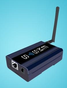
EMSYS Mini Gateway (SRV-1100) is primarily designed to to Wireless bridge. It is also an application server which means that it allows direct access to the collected data through a variety of interfaces.
